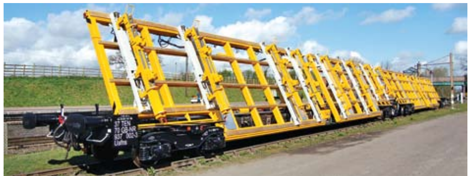
Hardware to implement Network Rail's 'seven-day railway' plan is becoming available. The first trestle wagon pair to carry pre-fabricated pointwork for on-site installation has arrived in the UK from Germany. Ian Allison
